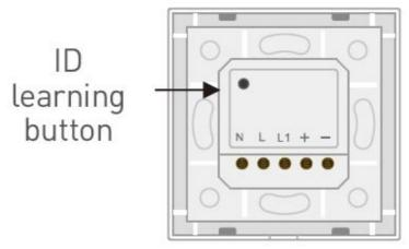
Long press the "ID learning button" on E61 for 10s until the lamps flash 5 times, clear code successfully.
