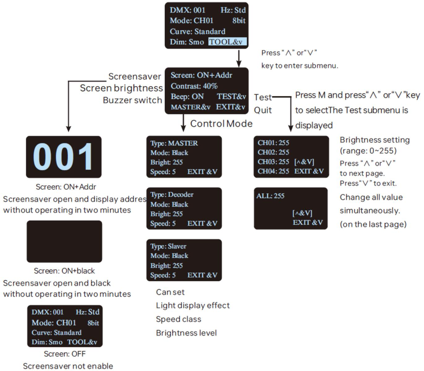
\* Fast self-testing function: press "A" or "V" keys simultaneously for 2-3 seconds under any page, decoder will enter self-testing function
