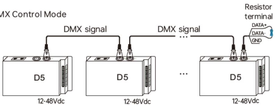
If the recoil effect occurs because of longer signal line or bad line quality, please try to connect 0.25W 90-120Ω terminal resistor at the end of each line
