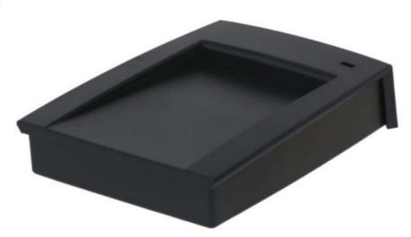
The Enrollment Reader is a plug-and-play device that connects to the PC through a USB cable. It can issue IC or ID cards. To achieve the best working condition of the device, please use the device flat on the table;e, do not place the device vertically on the desktop.
