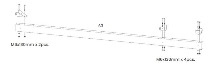
**b.** Build 6 spring hooks as per the diagram and turn the beam around to the right direction for next assembly step.
