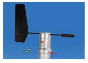
Finally, mount the sensor on the mast, orient the red nose to NORTH and tighten the screws (indicated by the arrow).
