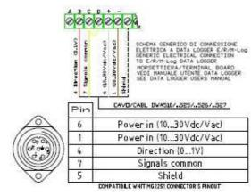
• If instead the DNA212.1 sensor replaces the DNA212 sensor, connect the existing cable to the new sensor using the CCDCA0004 adapter.
