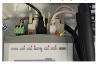
3. Within about two minutes the Signals Driving Unit turns on; this does not happen if the system is probably set to use the low power mode OMLP. To exit this mode, press the button on the top panel of the Main Power Unit
