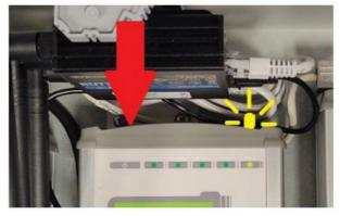
2. After a while, the Main Power Unit turns on, confirmed by the lighting of the green and red LEDs.
