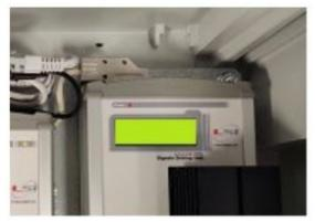
4. At the same time, the modem/router power is also activated, indicated by the green LED lighting at the Modem icon of the Power Unit panel. The modem/router may still be on if its power supply has been preset in a fixed way, without necessarily activating the corresponding section of power from the Power Unit.
