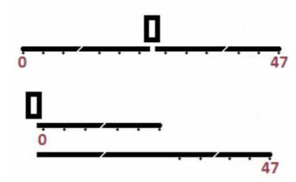
The figure shows the two types of installation of G.Re.T.A. concerning the electrode lines: G.Re.T.A. in a central position, and G.Re.T.A. in a head position. The LSI LASTEM after-sale team, based on the first measurements and the characteristics of the soil, will optimize the current injection parameters as well as those of the inversion algorithm for the specific site.
