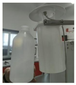
5. Fill in distilled water (PH: 5..7) inside the bottle and fix the bottle inside the sensor again. Reliable measurements will be available after 3-5 minutes. To confirm that the water has reached the temperature sensor, wrap the bulb in a thin layer of paper tissue and apply light pressure. If the tissue becomes wet, it indicates that the water has successfully contacted the sensor.
