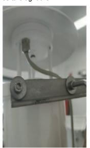
4. Unscrew the water tank from the sensor.
