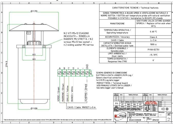
DMA122.1 sensor schematic drawing
