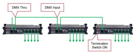
Recommended method of cascading multiple DMX splitters
