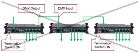
Connecting output to input is NOT recommended
