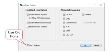
Houston X can now find the Mantra Mini or NEXEN using the old port number. Now use HOUSTON X to install the latest version of software in the Mantra Mini or NEXEN. See section 5.2. Installing the latest software changes the port number used by the device to the current port number. Next, un-tick the "Use Old Ports" box.
