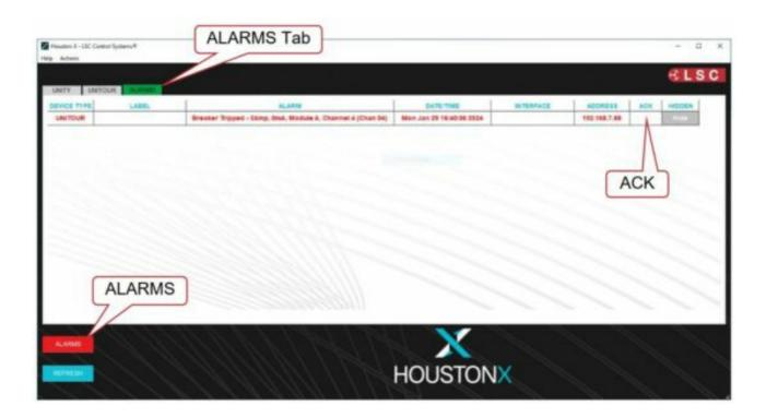
The alarm shows the device name, channel name, time and date of the fault along with a description of the issue.
