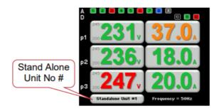
In standalone mode, the "Stagger Power On" times of the output channels are fixed to ensure that channels in different size APS units do not turn on at the same time.
