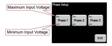
Pressing a Phase button allows you to select either the Low or High limit for that phase. These limits are also shown on the "Home" screen.
