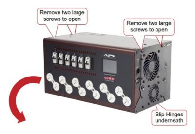
To completely detach the front section, remove the 4 large screws as shown then unfold the front section. Use a 10mm spanner to remove the 2 nuts holding the metal support straps and lift the straps off the bolts. Replace the nuts to retain the fibre washers. Carefully unfold the front section to the fully open position.
