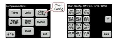
Each channel button shows its current configuration setting. Channels set to DMX show the DMX slot number to which they are patched.
