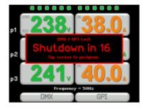
You can postpone the switch off and restart the countdown timer by tapping the screen. To disable the automatic switch off, set the "Power off delay" time to "Infinite".
