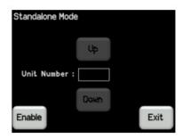
If multiple APS units are to be operated in Stand Alone Mode, you can prevent them from all starting their starting their staggered switch on sequence at the same time by assigning a different "unit number" to each APS. Each unit number adds an additional 12 second delay to the start of the staggered switch on sequence.
