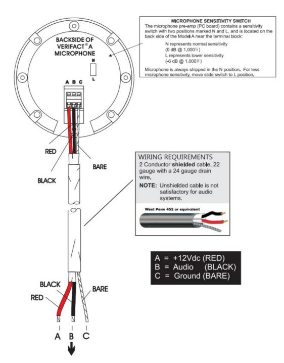
TO LOUROE BASE STATION OR TO OTHER LOUROE AUDIO RECORDING DEVICES (IF-1, IF-2, IF-4, IF-8 ETC.) CONNECTING A LOUROE MICROPHONE DIRECTLY TO AN IP CAMERA, ENCODER OR DVR WITH 3.5mm MONO AUDIO INPUT
