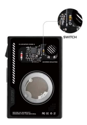
**Power On**: Press and hold the switch button for 5 seconds. The ringtone will sound and the indicator light will flash.
