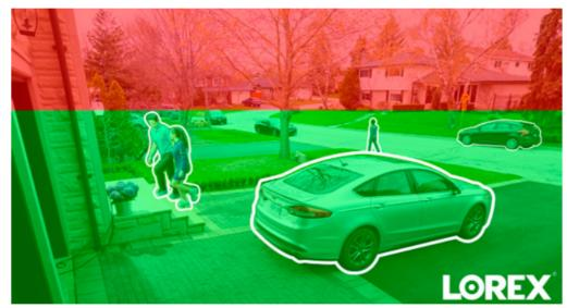
Lower accuracy for objects further away than 50ft ( $\sim$ 15m) and/or in the top  $\frac{1}{3}$  of the image. Optimal accuracy for objects within 50ft ( $\sim$ 15m) and in the bottom  $\frac{2}{3}$  of the image.
