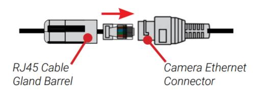
**NOTE:** The RJ45 cable gland is weather-resistant. Seal the cap with silicone and/or electrical tape for additional sealing if it will be exposed to precipitation regularly.
