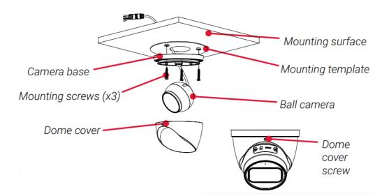
Use the included Allen key to loosen the screw on the dome cover. Do not loosen all the way.
