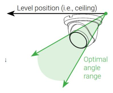
**NOTE:** Accuracy of person and vehicle detection will be influenced by multiple factors, such as the object's distance from the camera, the size of the object, and the height and angle of the camera. Night vision will also impact the accuracy of detection.
