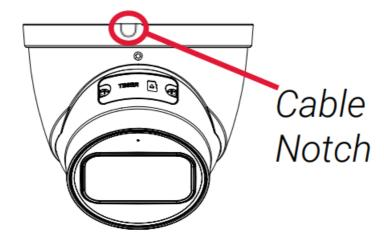
• If you run the cables along with the wall/ceiling, you must run the cable through the cable notch on the base.
