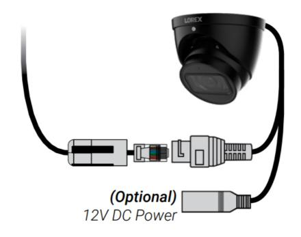
Connect the Ethernet cable to the camera.
