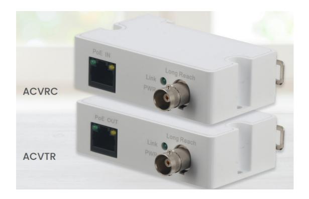
This product is divided into the transmitter (ACVTR) and receiver (ACVRC). Designed to work as a type of converter from RJ45 to BNC port, which supports long-range power supply transmission via coaxial cable adding convenience to expand your network security system. It provides one BNC coaxial port and one RJ45 port. For a reliable connection, this is equipped with two transmission modes that are 100Mbps and 10Mbps. Stay connected and be able to modify the transmission distance.
