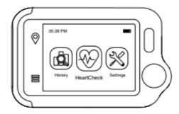
Press and hold the home button for 1 second to power on, and 3 seconds to power off.
