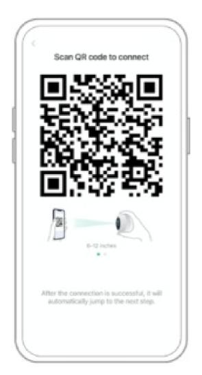
2. After pressing the camera switch for 3 seconds, the camera will turn on. At this moment, target the camera at the QR code of the mobile App, with a distance of about 20cm (about 7 inches) until the camera emits a "Di" sound, which represents the scanning is succeeded and the pairing is started.
