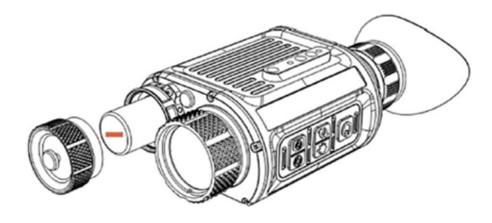
Figure 2.1 Battery Installation Illustrations
