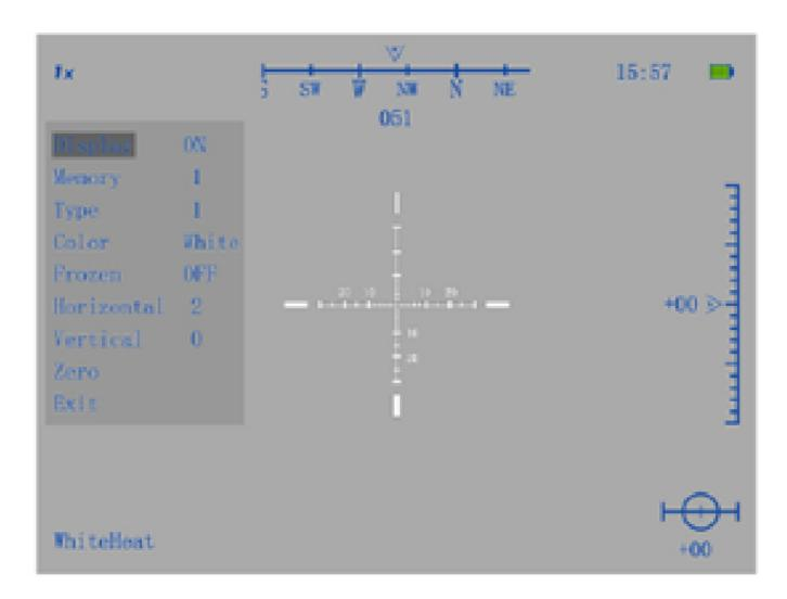
Set reticle display, reticle style, reticle color and reticle movement enable or disable.
