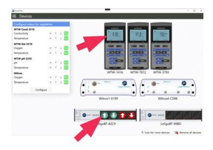
6. Each WTW probe and Witrox oxygen sensor must be calibrated before first-time use. See steps 12-14 for more information.
