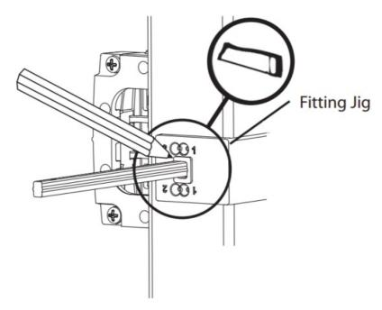
$6.\,$  Use file to ensure push rod is square and does not extend beyond post more than 3/16" (5mm).
