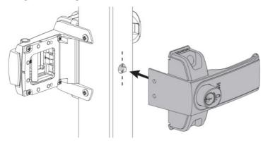
Firmly tighten screws on all components.
