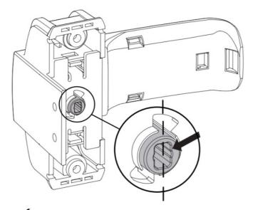
Ensure housing is in vertical position before fitting the Push Rod.
