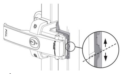
Adjust keeper so that the raised bump aligns with same on latch
