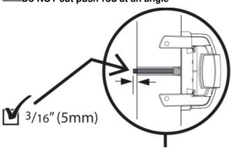
7. INSTALLING EXTERNAL ACCESS KIT (EAK)
