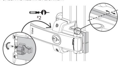
Adjust keeper so that the raised bump aligns with same on latch.
