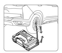
The inflatable hose is connected to the output port of the air inflate, and then tighten the nut, and the other end is connected to the car tire;
