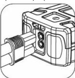
2. Connect the positive and negative of the clamps to the positive and negative of the car battery respectively, and make sure the connection is good.
