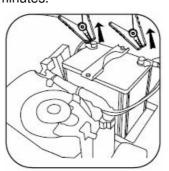
5. After use, please remove the clamps, and long press the "Power" button for 2 seconds to shut down, if the product is not operated for 60 seconds, the product will shut down automatically.
