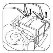
3. If the car starts successfully, the product will automatically turn off the power output of the clamps.
