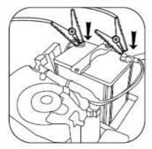
3. At this time, the green light on the main interface will flash, and the voltage of the Jumpstarter in parallel with the car battery will be displayed. After entering the start mode, if you want to only check the voltage of the car battery, short press the "Power" button to exit the start mode, the Jumpstarter will enter the measurement mode, and then the "green light" will go out, and the display only shows the voltage value of the car battery.
