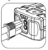
2. Wake up the product, short press the "LED light" button or short press the "Switch" button, if the connection is good, the green light on the display panel will be on and flashing, and the positive and negative voltages of the startup power supply in parallel with the car will be displayed at the same time. The car can be started at this time.
