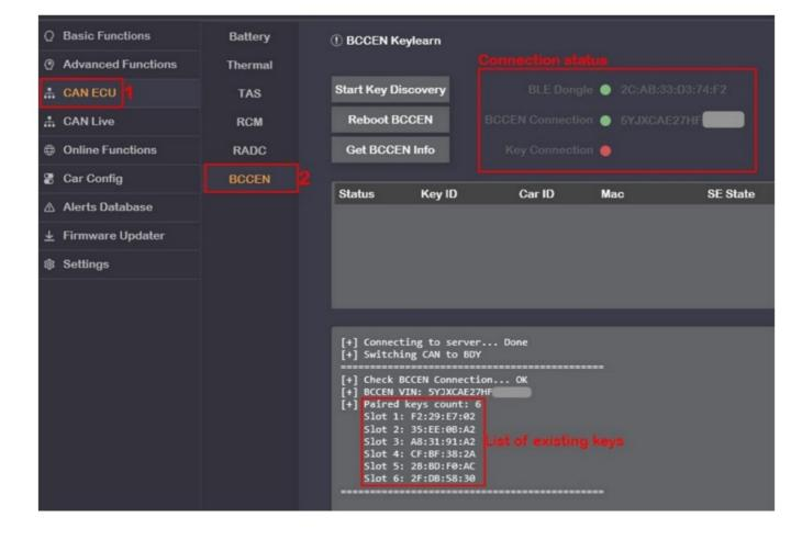
If the connection is successful, a list of keys in the BCCEN module and data about the vehicle and dongle will be displayed.
