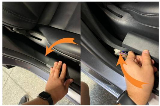
CAN VEH can be connected to the X930 connector located at the back of the center console.
