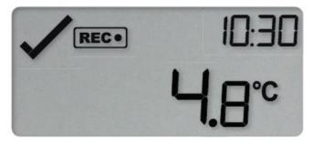
If no start delay was confi gured, the logger will immediately start recording. The logger should now be placed with the goods, so it reaches their temperature when the recording begins.
