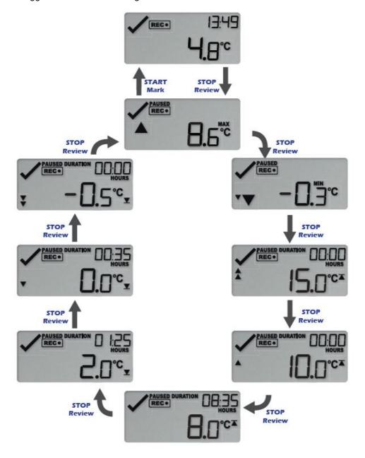
These screens show each confi gured alarm threshold temperature, and the time recorded during the trip above this temperature, in descending order. You can disable reviewing the alarm thresholds during confi guration of the logger. When the last review screen is shown, pressing STOP/Review shows the initial review screen again. If the START/Mark button is pressed at any time during the review, or neither button is pressed for 30 seconds, the or STOPPED screen is shown.
