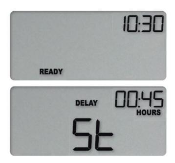
The display must show READY before the logger can be started. To start the logger, press the START/Mark button. If the logger was configured with a start delay, you will now see the DELAY symbol. The UTRID-16 starts a
