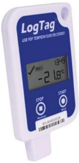
The LogTag® UTRID-16 is a fully confi gurable USB PDF temperature logger, which monitors and records the temperature of the surrounding environment and shows any alarm conditions on the built-in display. Alarm events can be reviewed on the display or downloaded to a PC via the built-in USB plug and analyzed using PDF soft ware such as Acrobat Reader.
