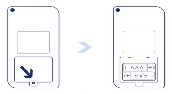
2. Once you have removed the battery cover, install the two AAA batteries. Take note of the direction each battery must be installed.
