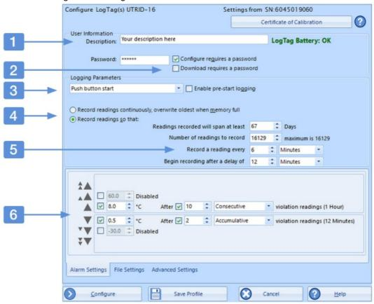
The top contains general parameters, while the bottom shows several tabs with additional settings.
