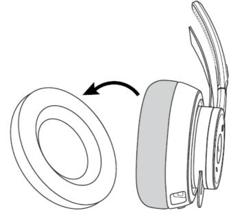
• Make sure not to pinch the foam cushion which can be damaged easily.
