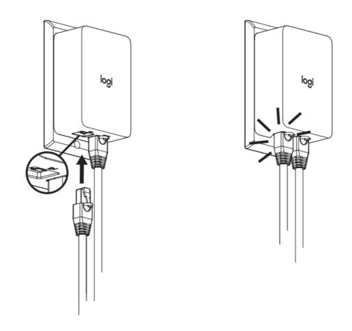
STEP 7: CONNECT THE OTHER END TO THE DONGLE TRANSCEIVER. PLUG THE DONGLE TRANSCEIVER INTO THE MEETING ROOM PC.
