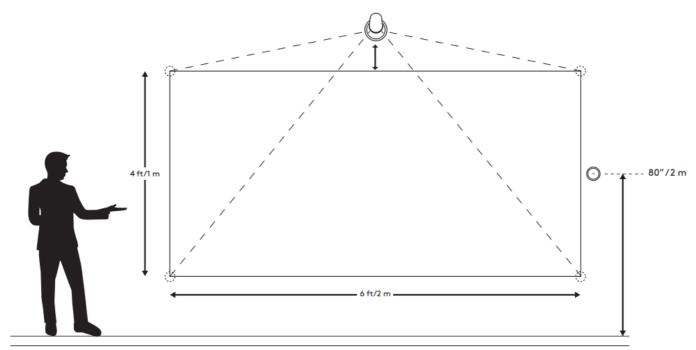
STEP 1: ATTACH THE CAMERA MOUNTING BRACKET
