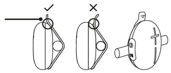
• ENSURE the hook is fully inserted into the hole in the speaker
