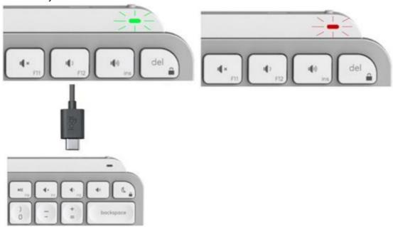
To charge, plug in the USB-C cable at the top right corner of your keyboard. You can continue typing while it is charging.
