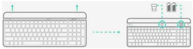
• Slide the upper part of the keyboard up to find the batteries and receiver storage inside.
