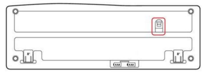
2. Slide the receiver into the slot.
