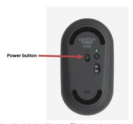
The power button is located on the bottom of the mouse. Slide the power button up to turn on the mouse.
