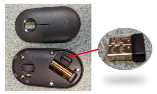
To USB Receiver is located inside the mouse. To extract the USB receive from the mouse, you will need to remove the top part of the mouse. The USB receiver is located inside the mouse next to the AA battery. Once the USB receiver is removed, you will need to insert it into your device's USB port.
