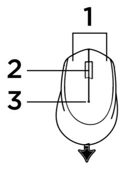
Flashes red when battery power is low. If the battery is not low, the LED indicator will turn green for 10 seconds when the mouse is switched on or after deep-sleep mode recovery.
