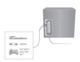
To use the RCA auxiliary input jacks on the rear of the subwoofer, plug your Logitech Squeezebox, DVD player, or game console into the RCA jacks using a 2-channel RCA cable (not included).
