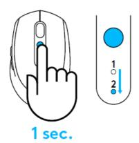
5. Short press Easy-Switch button to switch to next channel
