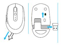
2. Remove pull tab or make sure your mouse is on and extract Unifying receiver from battery hatch
