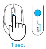
3. Short press Easy-Switch button to select desired channel
