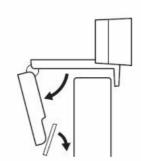
Adjust the webcam to make sure the foot on the universal mounting clip is flush with the back of your device.
