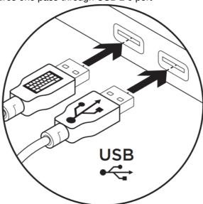
You must connect both USB cables in order to use the pass-through USB port
