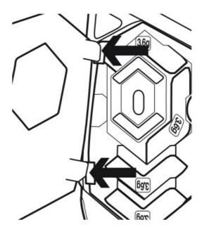
After inserting the weights, close the weight door by inserting the tabs on the weight door into the slots on the left side of the mouse and rotating the door down until the magnet holds the weight door firmly closed
