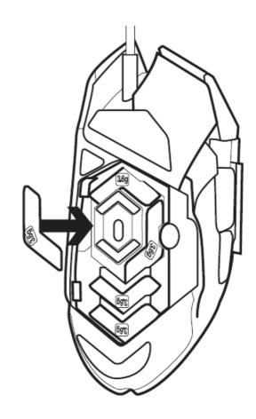
After inserting the weights, close the weight door by inserting the tabs on the weight door into the slots on the left side of the mouse and rotating the door down until the magnet holds the weight door firmly closed.
