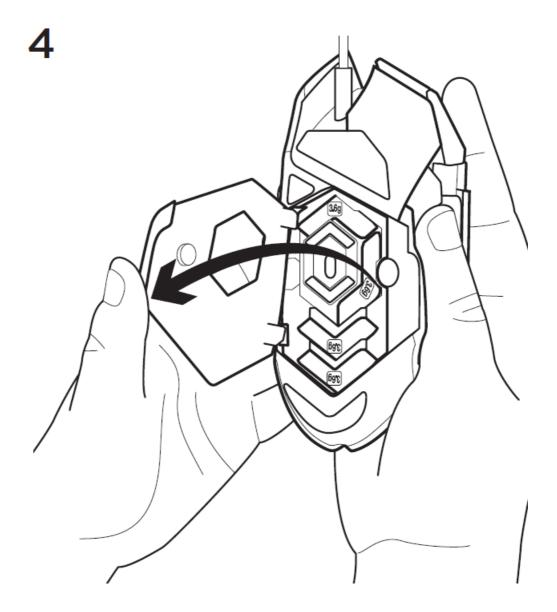
You can place up to five 3.6 gram weights in a number of different orientations. Experiment with different positions for the weights to find an overall weight and balance that feels right for you.
