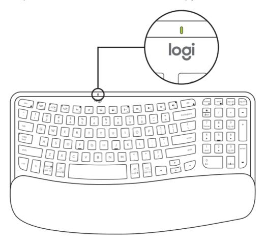
• 1b. When the battery level is below 6% (from 5% and below), the LED will turn red. You can continue using your device for up to 1 month when the battery is **low.**
