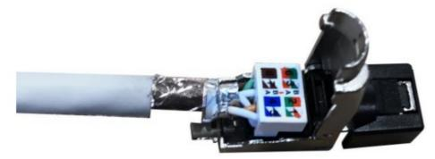
7. Place wiring cap on plug
