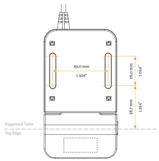
Fig. 4: Drilling Template CBlpaddle B and C
