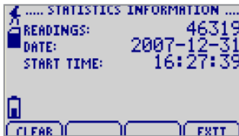
Type Statistics: Displays statistics from the pressure channel
