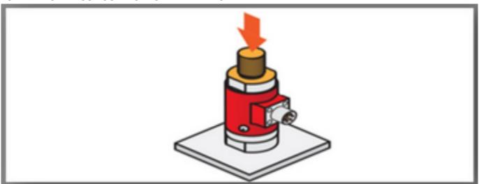
INSTALL IN A DRY, CLEAN ENVIRONMENT, UNLESS IP RATING ALLOWS FOR OTHER ENVIRONMENTS
