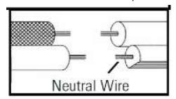
Twist plastic wire connector(D) until wires are tightly joined together ,wrap each connector with approved electrical tape for more secure connection, then carefully stuff all wires into the outlet box
