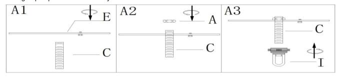
Step A2:Thread the hex nut (A)onto the nipple (C) till snug,.
