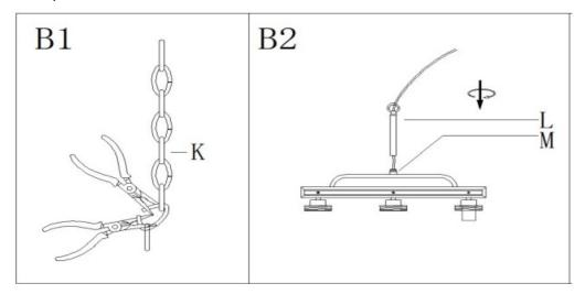
**Step B1:** By measuring, determine the correct number of links needed for proper hanging height. Using the chain pliers, disconnect and discard the remaining chain.
