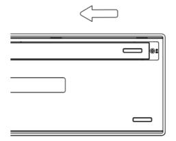
4. Insert the 2.4G receiver into the USB port of the computer
