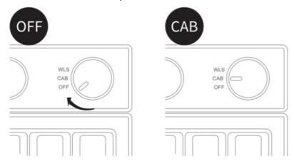
2. Take out the Type-C cable that comes with this product, connect the keyboard with device to complete the wired connection.
