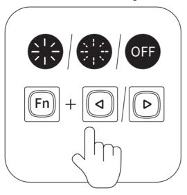
2. **2.Fn+**†/↓: Adjustment of backlight brightness.
