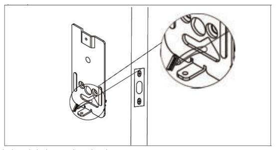
2. Route cable through the bottom of mouting plate.
